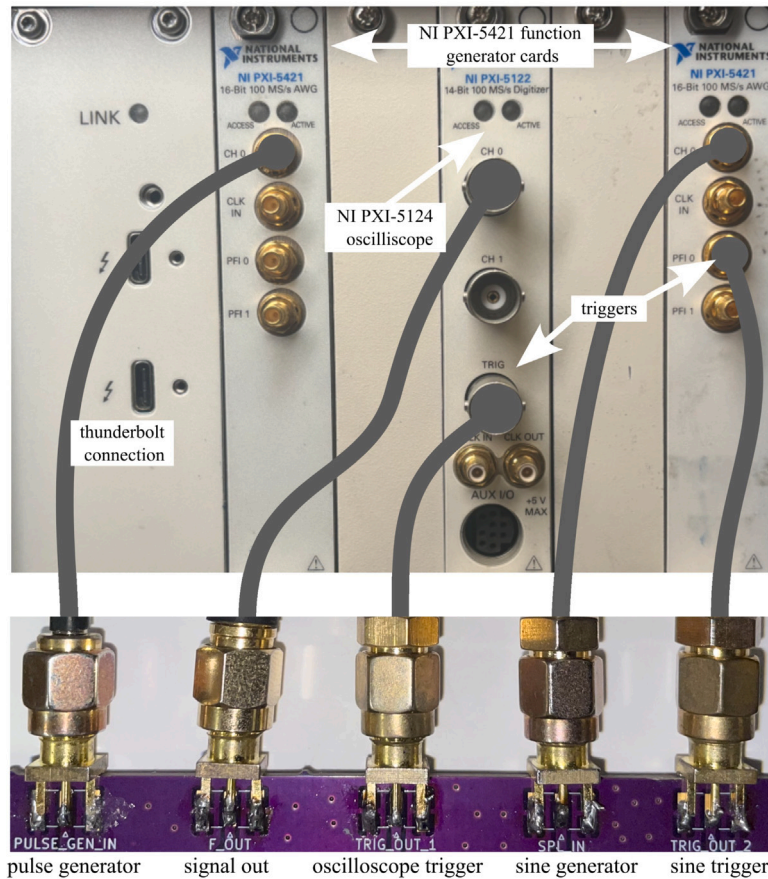
Fig. 18. Wiring diagram from the PXI cards to the control board.
