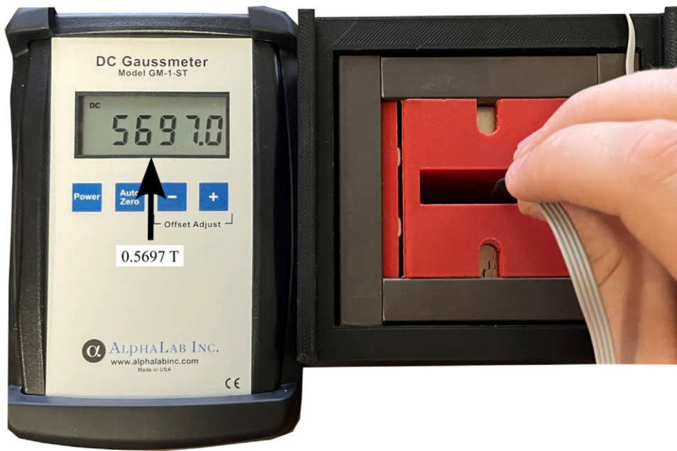
Fig. 13. Recording magnet inductance using a Gaussmeter.
